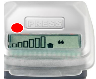
Display indication in case of dryness alarm (empty bars)
