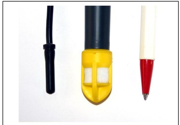
The absorbent material used is a special felt which is chemically inert and remains stable in the soil even after a long period of use. It also acts as a very effective filter so that only filtered water can reach the sensor. Due to small volumes of 1-2 cm<sup>3</sup>, it is also guaranteed that after a change in the fertilizer content, this can be detected very quickly in the jacket as well.
